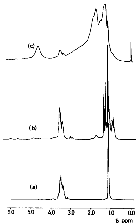
Figure 2 1 H n.m.r. spectra of (a) prepolymer (PPG-1200), (b) peroxydicarbamate (PC-I) and (c) PDCHI- b -PPO copolymer 2
